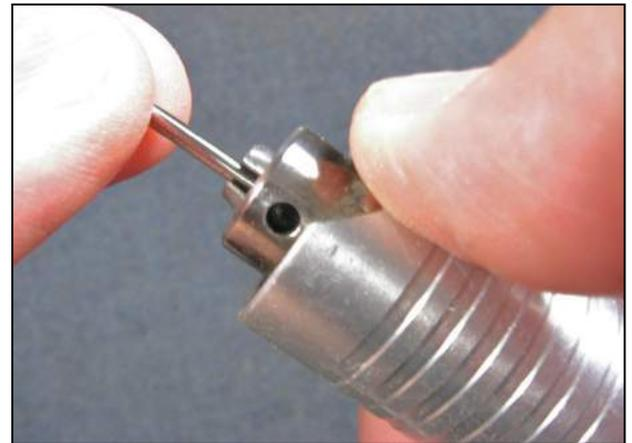
For closing the jaws around a smaller shaft, there's a neat trick. Hold the new bit in the center of the open jaws of the chuck, put your thumb lightly onto the outer toothed collar of the chuck, and gently start up the Foredom. As the chuck turns, it will naturally tighten the jaws around the bur shaft or the drill bit. Then all you have to do is a final tightening with the key.
